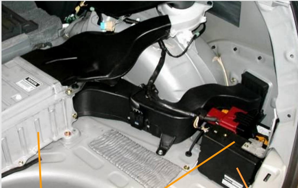
HV Battery (201,6 V)
