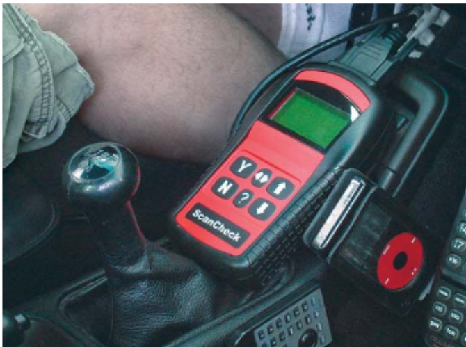
Figure 24-3. A scan tool is now the most important tool of the automotive technician. It will tell you where problems are located. (OTC/SPX Corp.)
