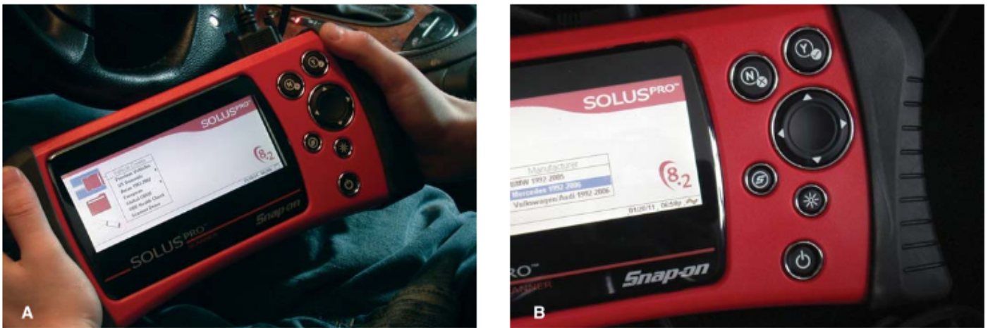
Figure 24-10. Always read the operating manual fully before attempting to use any model of scan tool. A—Scan tool controls vary from one manufacturer to another. B—Note the simple yes-no buttons that allow the user to quickly respond to the scan tool's prompts. (Snap-on Tool Corp.)
