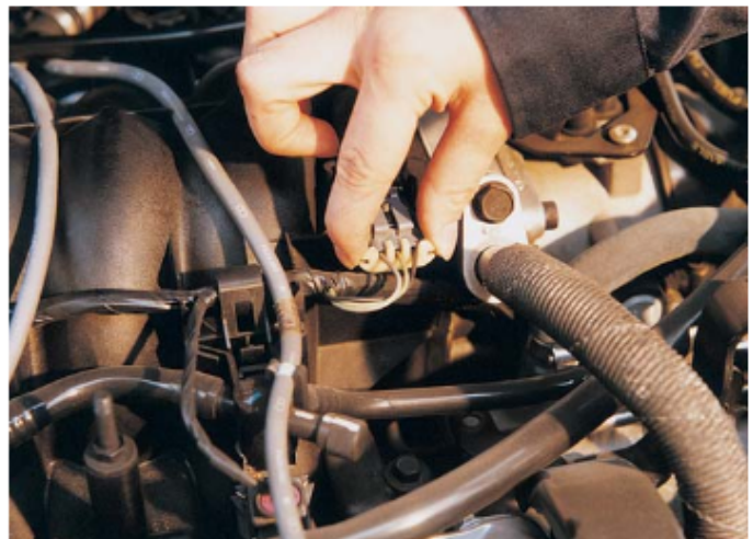
Figure 24-16. The wiggle test involves moving wires and connectors while scanning for trouble codes. If wiggling a wire trips a code, you found the location of the problem.
