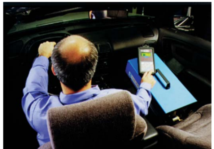
Figure 24-18. Scan tools are sometimes used while test-driving vehicles. This will allow you to check engine and vehicle operating parameters while duplicating the conditions present when the problem occurred. (OTC/SPX Corp.)
