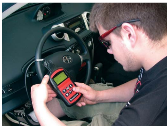
Figure 24-8. Once plugged into the vehicle, scan tools will quickly check the vehicle for stored trouble codes. (Snap-on Tool Corp.)
