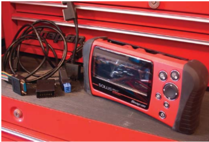
Figure 24-5. This advanced scan tool does not require cartridges. All important data for OBD II vehicles is stored in the memory. (Snap-on Tool Corp.)
