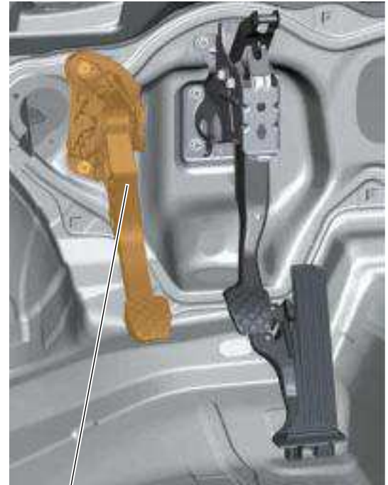
Clutch pedal with clutch position sender
