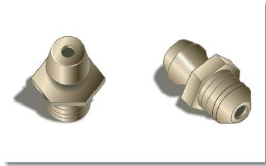
Grease fittings, or zerks, contain a one-way valve with a spring and a check ball.
