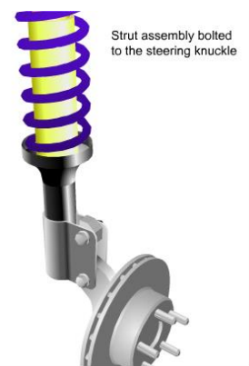
Strut assembly bolted to the steering knuckle.
