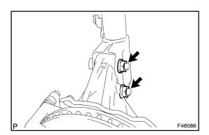
(d) Install the front shock absorber with coil spring to the steering knuckle with the 2 nuts.
