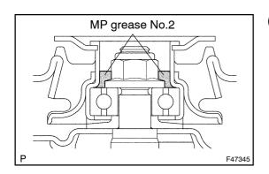
(c) Apply MP grease No.2 to the parts indicated in the illustration and install the front suspension support dust cover.
