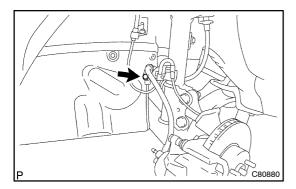
(e) Connect the front flexible hose No.1 and the speed sensor front LH to the shock absorber assy with the bolt.
