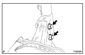
(b) Remove the 2 nuts on the lower side of the front shock absorber with coil spring.
