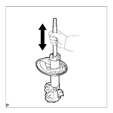
a. Compress and extend the shock absorber rod 4 or more times.
