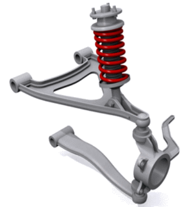
Double wishbone (Coil Spring type 2)
