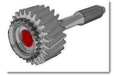
Note the roller bearings in this input shaft. The end of the main shaft rides on these bearings.
