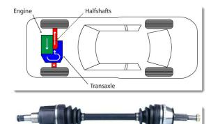
Halfshafts also must have greater flexibility than rear-wheel-drive driveshafts. Cardan-style U-Joints are restricted as a general rule to operation at angles of 15° or less. As a Cardan-style U-Joint's angle is increased, its reliability and its torque and speed capacity decrease proportionally. A different design is therefore needed when transmitting power and motion to a front wheel that may turn at a 30° or greater angle when steered.
