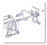
**Hydraulic Circuit** - Hydraulic clutches are very popular for several reasons, but they are by no means a new development. They are inexpensive to design, produce, and service, and hydraulics can multiply the force applied to the clutch pedal, reducing the amount of pedal effort required to disengage the clutch. Hydraulic lines require little space, and engineers can run them where convenient, so hydraulic clutches in a wide variety of different configurations can use similar components.
