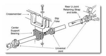
The two-piece driveshaft uses the same components as previously discussed, plus a center support bearing and slip yoke. Typically, the forward or transmission section of the two-piece shaft stays in position. The rear shaft accommodates all differential/suspension travel.
