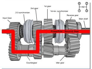
To shift into second gear, the first-reverse synchronizer moves into neutral, and then the second-third synchronizer moves to engage the second speed output gear. With the second speed gear now locked to the output shaft, a higher speed is attained, but with less torque increase than in first gear.
