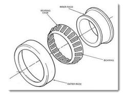
Rear axle bearings can be either ball bearings, straight roller bearings, or tapered roller bearings. Rear axles typically use tapered roller bearings to support the pinion gear and the differential case. Ball bearing or tapered roller bearings are used to support the axle shafts.
