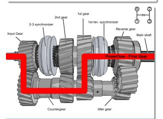
Shifting into first gear, the first-reverse synchronizer moves to engage with the first speed output gear. The other synchronizer remains in neutral. The first speed gear is locked to the output shaft and delivers high torque to the output shaft at low speed.
