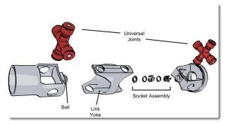
The center **link yoke** (which produces little vibration due to its light weight) becomes the only part that will still change rotational speed. Though better and smoother than a single U-Joint, the Double Cardan U-Joint only provides "near" constant velocity.
