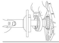
The front (input shaft) bearing for this transmission is a tapered roller bearing (right). The technician is installing the front bearing retainer or hub (left). In his other hand are shims and the bearing outer race. The shims are used to set shaft endplay.
