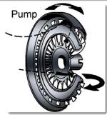
Note: As the vehicle begins to move, pump speed is greater than turbine speed. However, turbine speed will eventually reach pump speed. This means that transmission/transaxle speed will reach engine speed, and speed is no longer being converted in torque.
