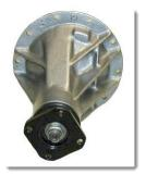
A separate yoke pressed onto the U-Joint caps is bolted onto the pinion flange for retention.
