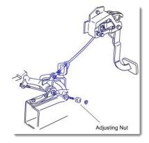
**Hydraulic Systems** - There is usually an adjusting nut on the fork pushrod, but sometimes it is located on the clutch master cylinder pushrod.
