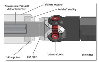
The slip yoke and transmission tailshaft are coupled using **splines** which allow the slip yoke to slide while receiving power from the tailshaft.
