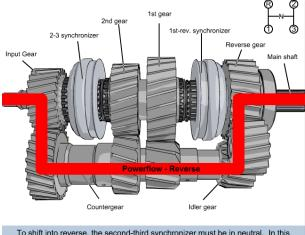
To shift into reverse, the second-third synchronizer must be in neutral. In this example, the first-reverse synchronizer moves into mesh with the reverse output gear, locking it to the output shaft. The countergear drives the reverse idler gear, and the idler gear drives the reverse gear backwards.
