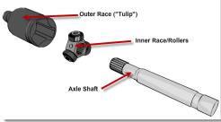
The **axle shaft** is splined to the inner race, which is retained by an external or internal snap ring. The outer race or tulip can have a **stub shaft** or **flange** made onto its outside end for attachment to the output shaft of the transaxle depending upon the specific vehicle's design.
