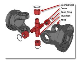
In the examples shown, the bearing cups are a precise fit inside the holes in the yokes. The cups are retained in the yokes by **snap rings**. These snap rings either fit in grooves machined inside the bearing cup holes or fit into grooves machined into the outside surfaces of the bearing cups themselves.
