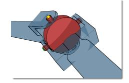
The main design limitation of Cardan-style U-Joints is that even when the driving yoke revolves at a steady, even speed, the driven yoke's rotational speed fluctuates. During driveshaft operation, the driving yoke stays at the same angle and as a result revolves at a constant velocity. The driven yoke changes angles as the rear axle assembly moves up and down on the vehicle's suspension. This angle change causes the driven yoke to speed up and slow down twice per driveshaft revolution.
