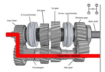
In neutral, both synchronizers are in their center positions. No output gears are locked to the main shaft, thus no power is transmitted. The input gear turns the countergear, but the output gears freewheel.
