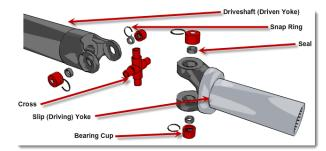
Some vehicles have driveshafts that are not designed to be field-serviceable. These have U-Joints that are staked or swaged in place. Some specialty machine shops or driveline shops can in fact replace worn or damaged U-Joints in these types of driveshafts.
