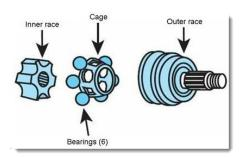
The **axle shaft** is splined to the inner race, which is retained by an external or internal snap ring. The outer race has a **stub shaft** made onto its outside end which is splined to the **wheel hub**. A **cage** fitted between the inner and outer race retains the bearings. The bearings connect and transmit power and motion between the inner and outer races.
