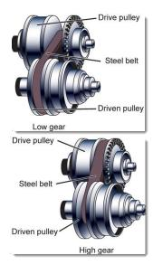
When each pulley is in the same position, the transmission ratio is 1 to 1.
