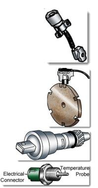
The manifold absolute pressure (MAP) sensor monitors the absolute pressure in the intake manifold and indicates engine load. In response to engine load, the PCM may delay upshifts or cause a downshift to provide extra engine power to the driving wheels.
