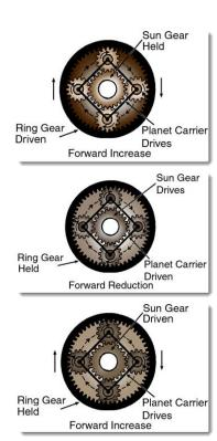
When the planet carrier is held, either the sun gear or internal gear can drive. With the planet carrier locked, however, a reverse movement occurs.
