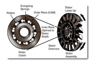
When the pump and turbine are turning at the same speed, the one-way clutch allows the stator to freewheel in the direction of the pump and turbine rotation. If the difference between the pump and turbine velocity is sufficient, the clutch will lock up the stator.
