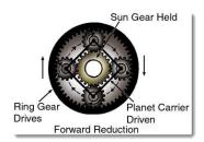
When the planet carrier drives and the sun gear is held, the planet carrier drives the ring gear. This arrangement produces a decrease in torque and an increase in speed through the ring gear.
