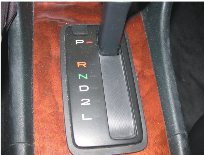
FIGURE 1-19 The gear selector is often called the “PRNDL,” pronounced “prindle,” regardless of the actual letters or numbers used.
