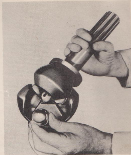
FIG. 7—ASSEMBLING UNIVERSAL JOINT BALLS
