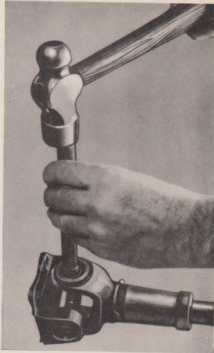
FIG. 3—REMOVING UNIVERSAL JOINT BEARING
