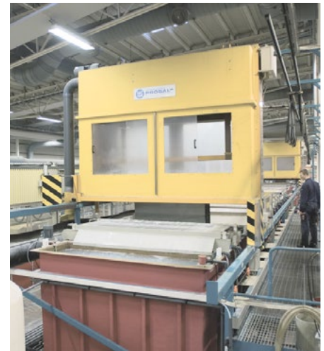
Automatic pre-treatment of enclosures before powder coating.
