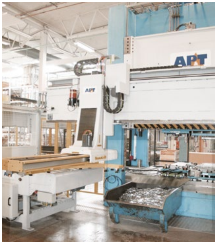
Fully-automatic plant for pressing, punching and bending of metal plates.
