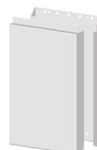
CDCA-CD Cable protection duct for fibre optic cables, for example (in CDCA). - Max cable diameter 25 mm inside cabinet. - Max. diameter for optical fibre pipes is 45 mm. - Degree of protection IP34D.
