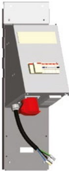
KSMUB 16/32 1x16 + 2x10 A or 1x32 + 2x10A with residual current device, miniature circuit-breaker and space for a kWh meter. Strength of short circuit 6 kA in combination with equipment max 63 A.
