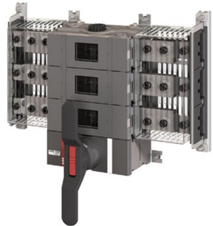
LBOD 1600 Section switch disconnecter without fuse up to 1250 A. To be mounted on Kabeldon IP-system. Degree of protection IP2X.
