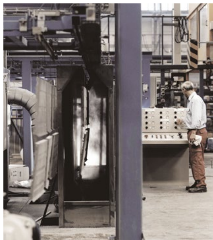
Powder coating of foundation parts.
