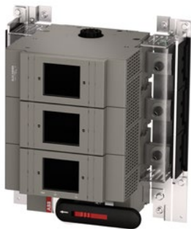
SLOC 630 Section switch-fuse with breaking on both sides of the fuse. 3-pole breaking with sealing possibility. System always dead when replacing fuses. Degree of protection IP2X.
